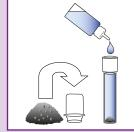
Weigh in your sample and add it to the extraction tube. Then, fill the tube with extraction buffer until the fill level.
