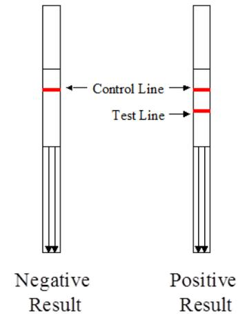
At least one line, the Control Line, should always develop. A red line in this position indicates that the strip is functioning properly. If the test strip displays 2 red lines, the test is complete and the sample is positive for *Listeria* species.
